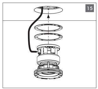
Add the appropriate number of speaker shims and install the speaker. Connect the negative wire to the black spring terminal and the positive wire to the red spring terminal.
