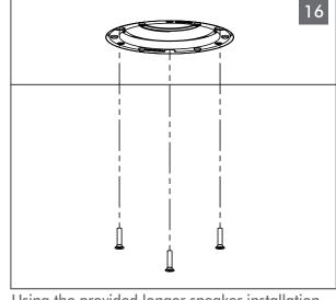
Using the provided longer speaker installation screws, apply Loctite to screws and screw speaker to mounting platform.
