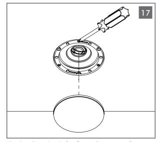
The leveling ring is for fine adjustment. If necessary adjust the magnetic grille leveling ring with a screwdriver and install magnetic grille. See grille painting instructions.
