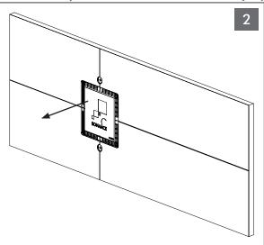
Remove the paint shield by pulling carefully. The back of the paint shield has adhesive. Save for later use!
