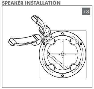
Remove the sanding shield support.
