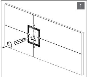
Using a philips screw driver, remove the sanding shield and set aside for later use. Discard the removed screw to replace with the longer 3/4" screw provided.
