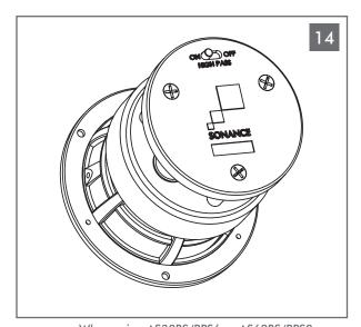
When using AS38RS/BPS6 or AS68RS/BPS8 System, switch to high pass ON. High pass switch is located on the back of the crossover cover. Switch high pass to OFF when choosing full range and no BPS6 or BPS8.
