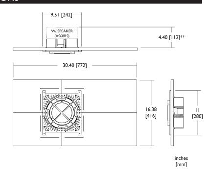
\*\* Depth from back of finish material to back of AS38RS speaker.
