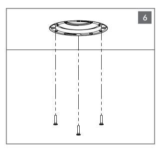
Apply Loctite® to screws and screw speaker to mounting platform.
