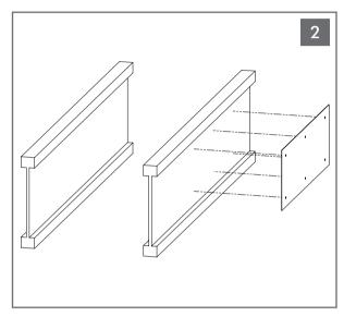
Place the mounting template on the side of the joist and drill six 1/2" (12.7mm) holes through the joist at the locations shown on the mounting template.
