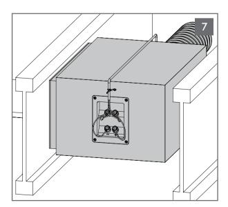
Secure the wires to the included zip tie near the terminals to prevent accidental removal by another tradesperson.
