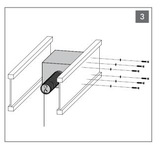
Hold the side of the BPS with the rubber damping pad up against the side of the joist and install the six lag screws and washers to secure the BPS in place.
