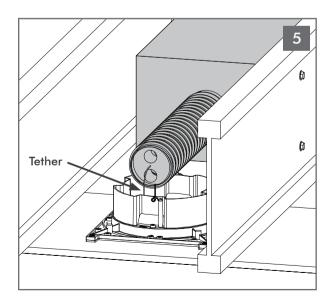
On the end of the BPS8 port tube there is a tether. The tether will be used later to guide the BPS8 port tube through the mounting platform opening.
