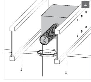
Attach the flex bracket to the joists. The flex bracket must be located within 12" (305mm) of the BPS8 to allow the port tube to reach through the flex bracket opening.
