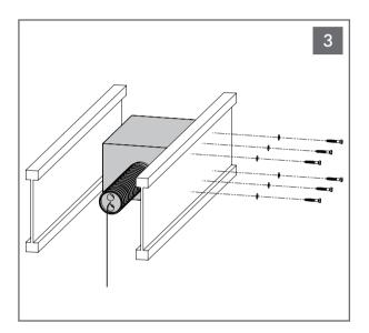
Hold the side of the BPS8 with the rubber damping pad up against the side of the joist and install the six lag screws and washers to secure the BPS8 in place.
