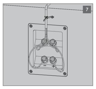
Attach the **four conductor wires** from the amplifier to the input terminals on the end of the BPS. Positive wires to red terminals and negative wires to black terminals. Run the speakers wires to amplifier location and run signal test with 9V battery. **NOTE: Port tube contains foam plug with tether, make sure pressure levels don't expel the foam and tether. Do not connect the voice coils in parallel.**
