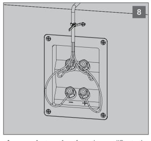
Attach the **four conductor wires** from the amplifier to the input terminals on the BPS8. Positive wires to red terminals and negative wires to black terminals. Run the speakers wires to amplifier location and run signal test with 9V battery. **NOTE: Port tube contains foam plug with tether, make sure pressure levels don't expel the foam and tether. Do not connect the voice coils in parallel.**
