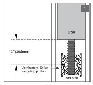
Determine the location for the mounting platform. Ensure there is adequate room for the BPS8 subwoofer at the location of the platform. The speaker opening must be located within 12" (305mm) of the BPS8 to allow the port tube to reach through the platform.
