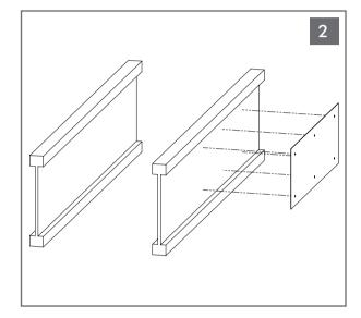
Place the mounting template on the side of the joist and drill six 1/2" (12.7mm) holes through the joist at the locations shown on the mounting template.
