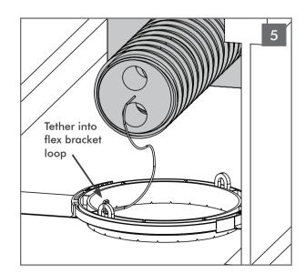
Loop tether into the flex bracket. Pull tether all the way until port tube lies firmly on the flex bracket. Tie tether into a knot. This process ensures that other tradespersons won't infringe on port tube assembly area.
