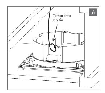
Position end of port tube as close as possible to back of mounting platform. Loop tether into the anchored zip tie and secure. This process ensures that bandpass connector is easily attached later and other tradespersons won't infringe on port tube assembly area.
