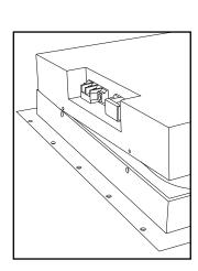
Position enclosure to the side of the IS speaker, connect leads to the enclosure.
