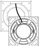
Attach the woofer driver to the enclosure using the twelve hex head screws. The appropriate hex driver is included with the screws.
