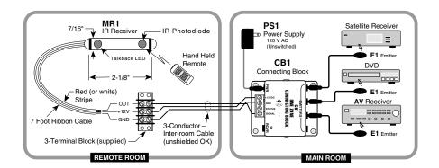
While it is possible to make wired connections without the connecting block, it is not recommended. The connecting block reduces installation time, helps to eliminate errors, allows easy troubleshooting, and permits easy system upgrades later, if needed.
