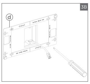
Using the recommended screwdriver and (d) mounting screws, install the first screw in the upper left-hand corner.
