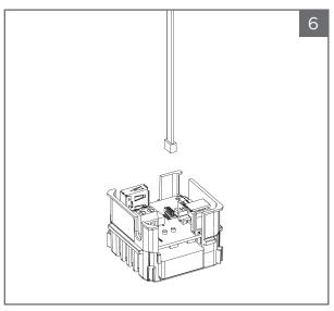
Connect the (a) bezel's serial cable to the serial port found on the (f) PoE splitter.
