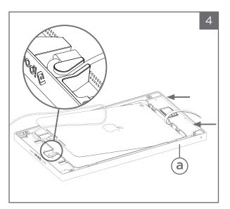
With the (a) bezel face down on a flat, non-scratch surface with the iPort logo on the right. Plug in the iPad's lightning to USB cable directly into the iPad. Position the iPad facedown into the (a) bezel with the iPad cable on the right. Wrap the iPad cable around the (a) bezel's metal loop. To lock the iPad in place, use a flat head screwdriver to deploy the two toggles located on the right side of the (a) bezel.
