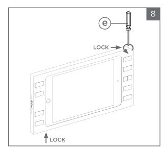
The Surface Mount will attach to the (b) mounting bracket with internal magnets. To lock the Surface Mount in place, use the (e) security tool provided to engage the security locks. When the bezel is in landscape orientation, the security holes are located on the top-right and bottom-left of the bezel. Rotate the (e) security tool counterclockwise to engage the locks, and clockwise to unlock the Surface Mount (a) bezel from the (b) mounting bracket.
