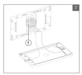
Connect the appropriate power source identified in the Power and Wiring Guide (found in (f) PoE splitter box). Place the PoE splitter into the single gang box located in the wall with the iPort logo facing out. NOTE: If you need to remove the (f) PoE splitter from the wall box, you can use needle-nose pliers to grab onto holes provided on the front of the (f) PoE splitter.
