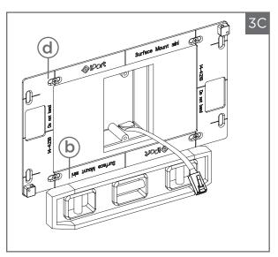
Level the (b) mounting bracket over wiring location and fasten (b) bracket with the remaining (d) screws. Lining up the (d) mounting screws with the engraved center lines provided on the (b) bracket will allow you optimal adjustability. The (b) mounting bracket is now in place.
