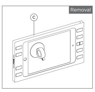
The (c) suction cup (provided) is used to remove the iPad and (a) bezel from the (b) mounting bracket. Once the (a) bezel is unlocked from the (b) mounting bracket, depress the (c) suction cup on the corner of the iPad screen and carefully pull the iPad from the wall, while the other hand is supporting the opposite side of the (a) bezel.
