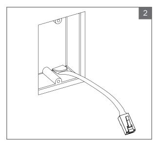
Locate the ideal mounting area. For retrofit installation, locate an existing low-voltage electrical box. For new construction, choose a location for an electrical box. We recommend installing the (a) bezel in landscape orientation, but it can also be installed in portrait orientation, NOTE: A single gang electrical box allows you to use the Surface Mount in portrait or landscape orientation, and a double gang electrical box allows you to use the Surface Mount in a landscape only orientation.
