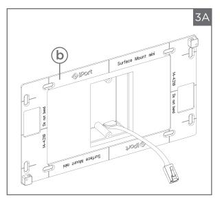
Install the (b) mounting bracket on the wall with the (b) bracket surrounding the electrical box. Use the center lines as a guide to install the (d) mounting screws. Our specialized (d) mounting screws act as anchors and screws when mounting on a drywall or wood surface. NOTE: Glass mounting is not recommended for this product.
