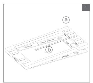
When removing the Surface Mount (a) bezel from its box, the bezel will be attached to the (b) mounting bracket. To decouple the (a) bezel from the (b) mounting bracket, place the (a) bezel face up on a flat and smooth surface. With one hand, hold the (b) mounting bracket in place. With your opposite hand, lift the right edge of the (a) bezel and then the left to decouple the magnets. This will help avoid bending of the metal, and prevent any damages to the (a) bezel or (b) mounting bracket.
