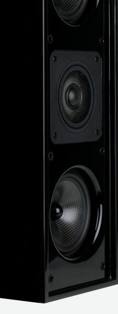
Sonance Cinema Living speakers are constructed from the highest quality materials including carbon fiber and Rohacell® laminated or polypropylene speaker cones, silk dome ferrofluid-cooled tweeters, die-cast aluminum baskets and 3/4" medium density fiberboard enclosures.
