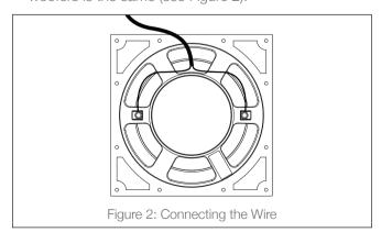
3. Attach the woofer driver to the enclosure using the twelve Phillips head screws.
