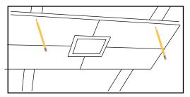
Prior to attaching the panel bracket to the framing material, position the mounting platform in the desired location - do not fasten at this time. Mark the center of the framing material on the frontside of the panel bracket.
