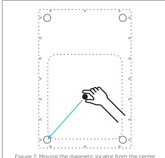
Figure 2: Moving the magnetic locator from the center of the woofer location to the lower left embedded disc.
