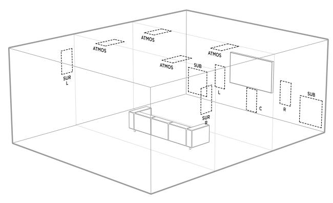
**NOTE:** Center channel can be oriented horizontally for space savings. Place tweeter on center line of room for best performance. Custom framing required due to >16" speaker width.
