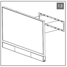
Carefully mount display & Soundbar to wall bracket. NOTE: When lifting, be careful not to place too much pressure on, or twist, the Soundbar. This could bend the bracket.
