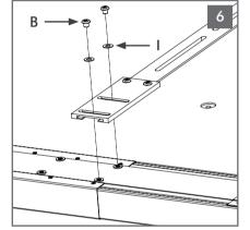
Position Soundbar as close to display as possible. Firmly fasten (B) screws & (I) washers to connect Soundbar to the Soundbar connectors.
