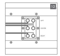
Complete wiring to Soundbar & display. If possible, leave enough wire out of the wall to allow for connection prior to mounting to wall bracket.
