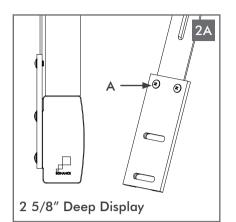
Choose & attach the correct Soundbar connector with (A) screws. The flat Soundbar connector will align with 2 5/8" (65mm) deep displays.
