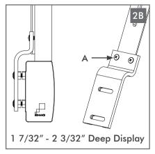
The recessed Soundbar connector will align with displays from 1 7/32" - 2 3/32" (31.74mm -53mm) deep. Use (C) or (D) screws and (G) nuts.
