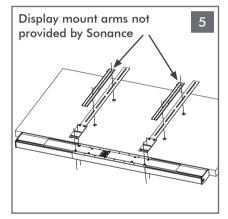
Place attachment rails on display & Soundbar making sure that holes and rails are aligned.
