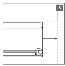
Loosen screw to allow for adjustment of Soundbar grille. No tool required.
