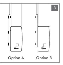
Alignment options for Soundbar: A) Top edge of Soundbar aligned with front of display. B) Front radius of Soundbar aligned with front of display.
