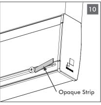
Cover open area with black opaque strip & cut to size. This will prevent any light from passing through grille.
