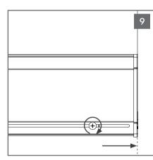
Slide grille to edge of display & tighten screw. No tool required.
