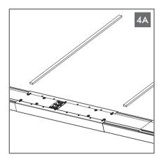
**Option A**: Use included 8mm display spacers. This creates the offset needed for bottom of display to align with top of Soundbar. Carefully place display on top of spacers. Be careful not to scratch front of display. Skip step 4B.
