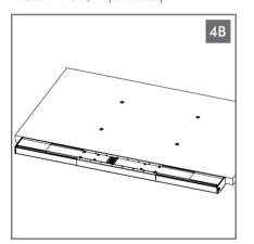
**Option B**: Lay display & Soundbar on same surface (without display spacers). Be careful to not scratch front of display.
