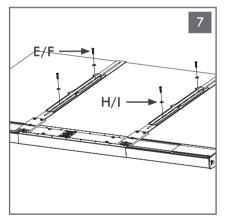
Install display wall bracket using spacers & screws supplied with display mount or (E)/(F) screws & (H)/(I) washers. Hardware will vary. It is recommended to keep spacers provided with display.
